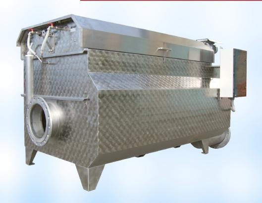
Microscreen drum filters are an ideal solution for the water from waste water treatment plants filtration. Here they are installed as the third, final level of water treatment. In case, the water treatment plant does not meet sufficiently the required outlet quality limits of filtered water, by introducing the microscreen drum filters the limits can be safely achieved.
